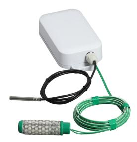
Wireless soil moisture logger is used to measure the amount of water in the soil. The sensor work with the Efento mobile application for Android and allow, among others registering soil moisture and temperature, notifications of a sharp decrease or increase in the amount of water in the soil, and generating automatic reports. The devices are powered by a battery that ensures their maintenance-free operation for a period of at least two years.
