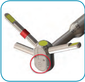
FlowTracker2 with optional integrated pressure (depth) sensor.
