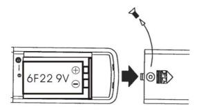
When the low battery symbol is displayed on the LCD, replace the old batteries with two new batteries.
