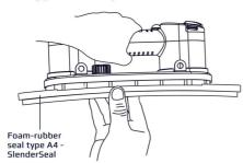
STEP 3 - Replacing a seal part Should the outer black foam seal of the Slender Seal system require replacement due to damage or wear and tear; remove the outer black foam seal and carefully press the replacement seal into place. Ensure the outer black foam seal fits snugly and securely before use.
