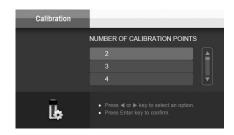
1. Press the **Cal** key to enter the calibration mode, the meter prompts to select the "Number of Calibration Points".
