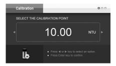
If necessary, press the ◀ or ► key to select desired calibration point (e.g., 10.00 NTU).
