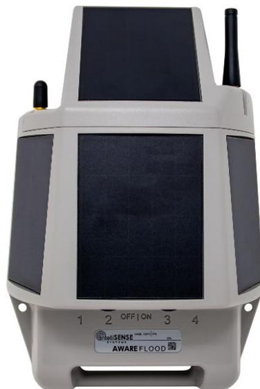
The AWARE Flood System is comprised of a network of sensor nodes, each consisting of an IoT sensor node that is connected to a submersible water level sensor through a 49-foot cable to independently monitor waterway conditions. Data from the wireless network can be sent via either a direct cellular Internet of Things (IoT) communications link or an Iridium satellite connection for reliable data transmission around the world.
