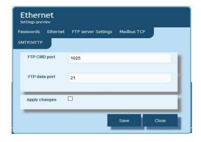
Fig.18 View of FTP ports configuration window
