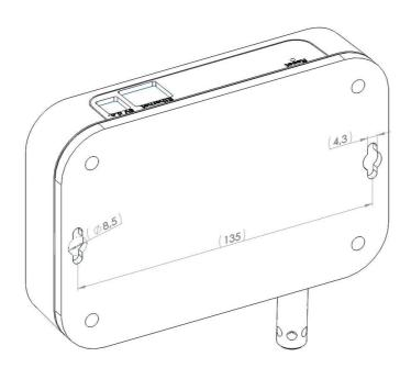
Fig. 2 Location of mounting holes
