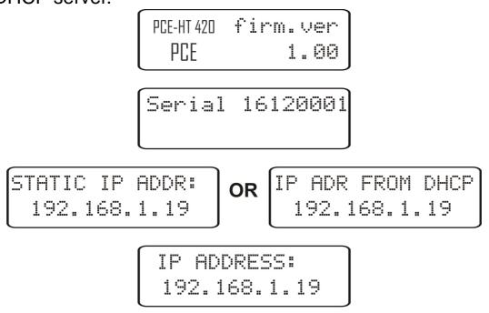
Fig. 4 Startup messages of PCE-HT 420 monitor
