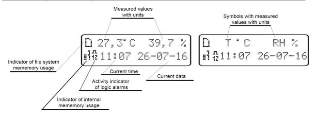
Fig. 5 Description of the monitor reading field
