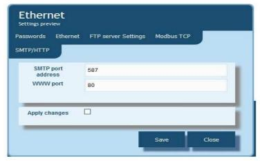
Fig. 20 View of SMTP port configuration window on "Ethernet" tile
