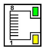
Fig.6 View and numbering of RJ45 slot pins
