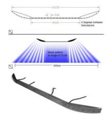
This 32-element transducer array was designed to cover a large section of seabed with high-resolution.
