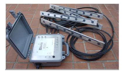
The SeaTek ultrasonic ranging system shown above is composed of 4, 8 element, stainless steel arrays, and an electronics package. The transducer spacing is 8 cm (center to center). All four arrays can be mounted to form a continuous 256 cm (8.4 feet) long array.
