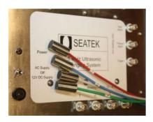
Our most popular and versatile transducer is the cylindrical transducer. They are housed in stainless steel housings and are 1 inch in height and 1/2 inch in diameter and are typically bundled four per cable.
