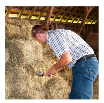
Hay hygrometer to determine moisture and temperature of hay and straw / Robust design / Four different lengths of measuring lance of 25 cm, 50 cm, 100 cm or 200 cm /
