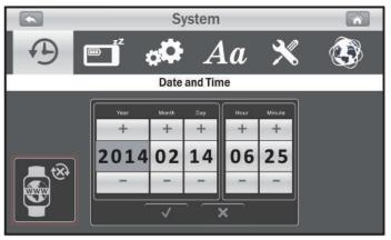
**NTP Clock:** Tap the icon  $\bigotimes$  to automatically synchronize system clock with a network Time Protocol(NTP) time server
