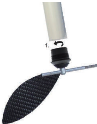
Figure 9.( Bearing replacement – Wind speed/direction sensor)
