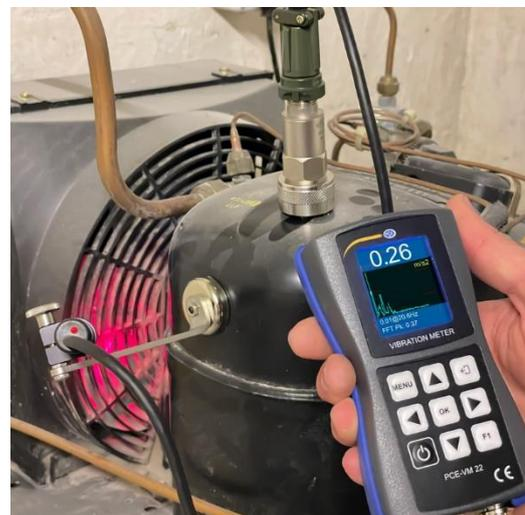
With the new vibration meter from PCE Instruments, not only vibration values but also RPMs and surface temperatures of components can be recorded immediately in the same device, making it particularly easy to assign them to the measuring spot and the time of measurement. This simplifies both the process of routine checks for preventive maintenance and the search for the causes of irregularities and deviations.
