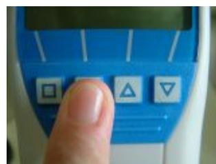
In the type selection menu the calibration curves can be changed by pressing
