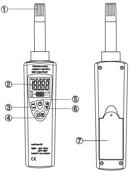
1) Humidity / ambient temperature probe: semi conductor sensor for humidity and temperature inside.
