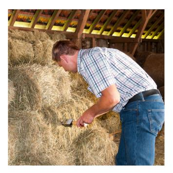
Hay hygrometerto determine moisture and temperature of hay and straw / Robust design / Four different lengths of measuring lance of 25 cm, 50 cm, 100 cm or 270 cm /
