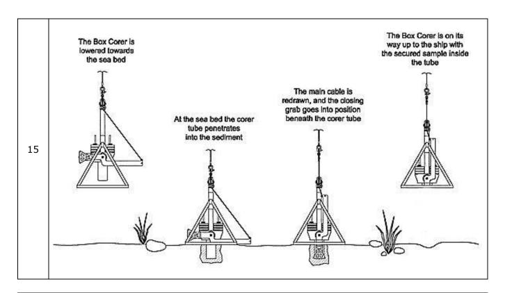
As soon as the box corer hits the seabed, the upper part releases from the main rack. Upon retrieval, the upper part will hold the box corer by means of the two 8 mm steel wires attached to the arms.
