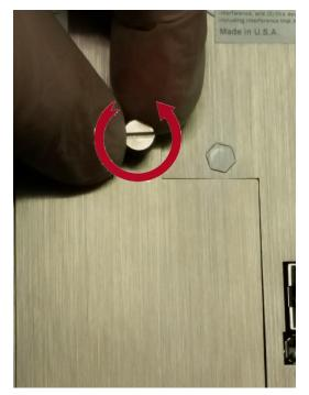
Step 1 – Loosen the Knurled Thumb-turn screw
