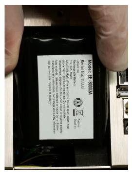
Step 5 – Carefully push battery into the compartment
