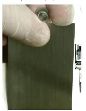
Step 2 – Remove Battery Compartment Door
