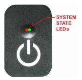
Unit plugged into AC (instrument screen on or off)
