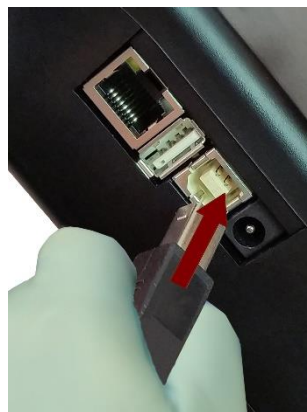
Connecting USB - B Client
